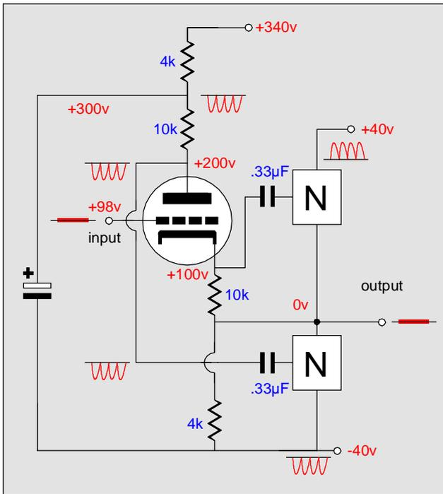
Reversing the connections to the phase splitter requires reversing our strategy. Now the phase splitter's cathode needs to see no noise and the plate needs to see the full negative power supply rail noise. The filter capacitor's connection to the negative power supply rail ensures the coupling of the rail's noise to the phase splitter's plate and, then via the coupling capacitor, to the bottom device's input.
