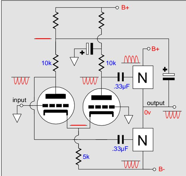
The circuit below shows the addition of the constant current source and the inversion of the noise at the output. What happened? The constant current source only shifted the source of the noise to the bottom device.
