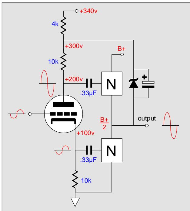
Split-load, plate-referenced, gain output stage
