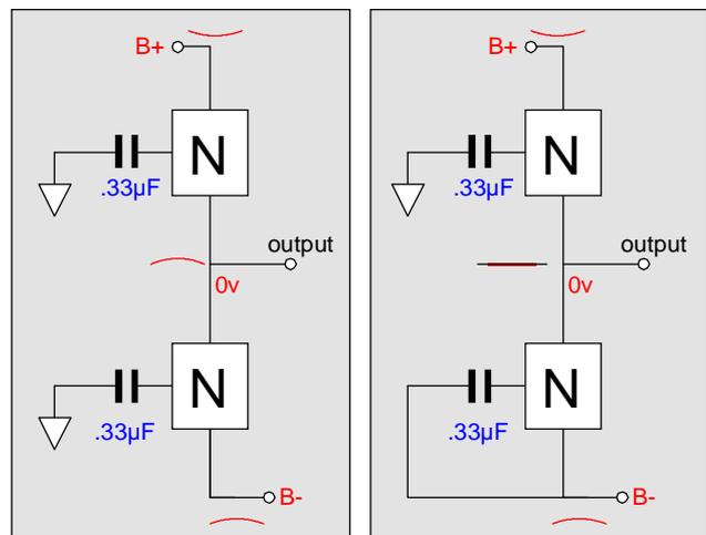
And if the amplifier does not use a global feedback loop, the sound will suffer. Unless, of course, we match the sagging negative rail voltage with a negative drive voltage. The circuit below shows the top device seeing the negative power supply rail noise reflected to its input, which will make it to the output. Is the answer to replace the cathode resistor with a constant current source?
