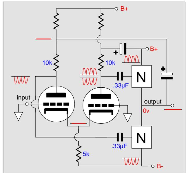
The cathode resistor's value must equal half the plate resistors value or the noise cancellation will not occur. Thus *the cathode resistor should not be replaced by a constant current source*. The same holds true for replacing the plate resistors with current sources. So the answer to the question, "Are current source a good idea in tube equipment?" is sometimes yes, sometimes no, and sometimes it makes no difference.
