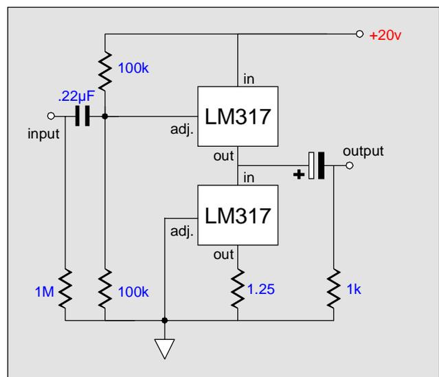
Thus the device decreases its conduction equal to its transconductance, if the idle current was high enough to absorb that amount that is; or it ceases to conduction altogether, if the idle current is not high enough. And a negative going pulse will provoke an increase in conduction equal to the transconductance of the device. This is classic follower action in a nutshell.
