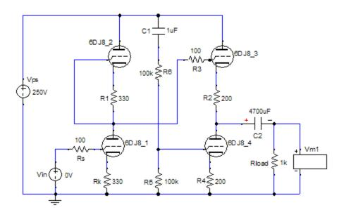
Above is a schematic of the circuit used in the  $B^2$  Spice A/D simulator. The idle currents were close with 8.22mA for the first stage and 11.88mA for the second stage.
