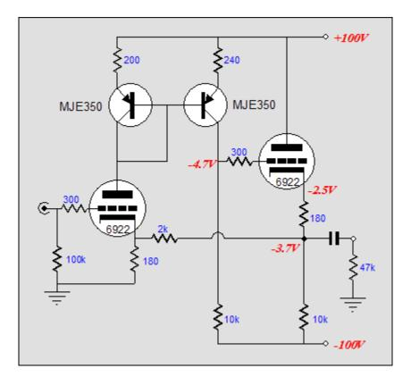
Since the output is in phase with the input, and since the amplifier puts out so much gain, a feedback loop is easily added and needed to bring down the gain to 8, which equals +18 dB (this more than enough, as +6 to +12 dB of gain is all that most line stages need).
