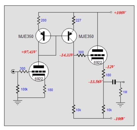
The entire amplifier (using 6922s and some tweaking) performs fairly well in simulation (real results may—and invariably do—vary).
