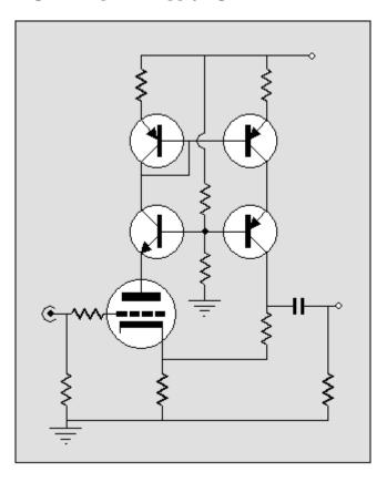
Still, the problem this topology faces is that it does not improve upon a grounded-cathode amplifier's PSRR. Inverting the cascode and adding a constant-current source will take care of the PSRR troubles, as the B+ noise cannot make across the constant-current source.
