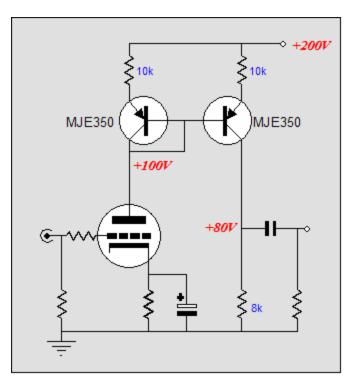
On the other hand, when the emitter resistors are low in value relative to the triode's rp, say 100-200 ohms, then the Miller-Effect capacitance disappears and the gain climbs close to gmRa.
