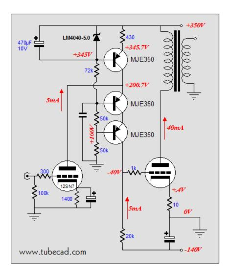
Two MJE350s are used in the cascode portion of the circuit, decreasing the likelihood that the high voltages with the amplifier will kill one of the fragile transistors.
