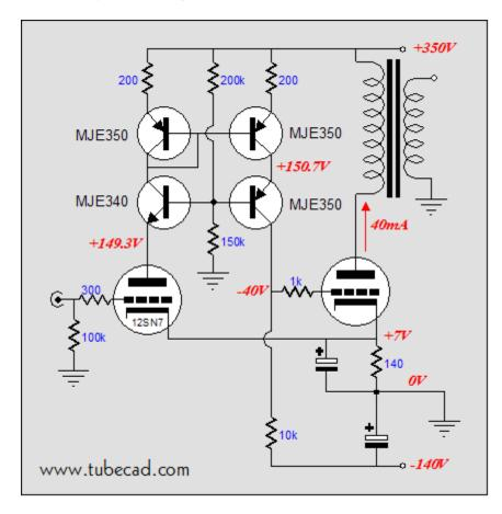
If the output tube draws too much current, the input tube conducts less, which decreases the voltage across the load resistor, which in turn decreases the output tube's conduction. The opposite situation is easy to imagine.
