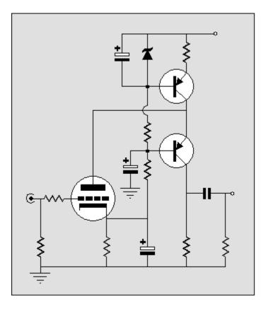
A truly low-noise cascode offers some real advantages for preamps and line amplifiers. One use for this circuit that comes to mind is that of an input stage in a single-ended amplifier.
