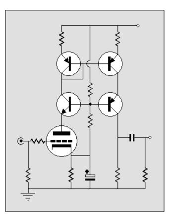
One advantage that immediately comes to mind is that we can now use lownoise, low-voltage transistors in the current mirror portion of the circuit. Second, we could use multiple PNP transistors in series to allow even high voltages to be used. Last, the cascoding would greatly improve the PSRR figure when used with a monopolar power supply, as the triode would not see any of the B+ noise on its plate.
