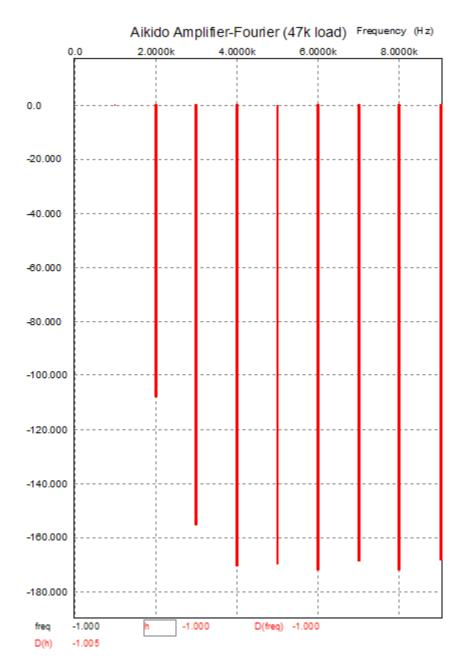
The winner is obvious in terms of distortion; both tie in output impedance; and the Aikido (using all 6922s) only has a gain Of 16 (+24 dB). What if we swapped some of the current-mirror-based amplifier's gain for linearity?
