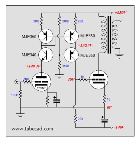
No tube is perfectly linear. All triodes are easier to turn on than they are to turn off. This make for a strong 2nd harmonic distortion component.
