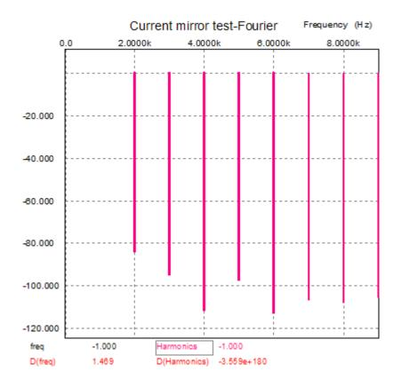
When using a transistor-based current mirror, I always match the transistors, believing it critical, besides my VOM holds a hfe test, which makes the matching painless. Well, using unmatched transistors, with one having twice the beta as the other, only slightly increased the distortion and reduced the current mirroring efficiency by less than one percent, so maybe I have been overly nervous.
