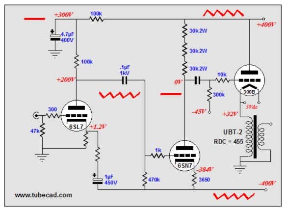
Alternatively, we could use a cascode input stage. Normally, the cascode is rightly viewed as having an appallingly low PSRR figure—in fact, virtually none. But in the totality of the entire amplifier circuit, this liability becomes an asset. All we have to do to exploit the cascode's poor PSRR figure is terminate its plate resistor into the negative rail, not the positive B+ nor ground. As shown below, almost all of the negative rail noise will appear at the cascode's output.
