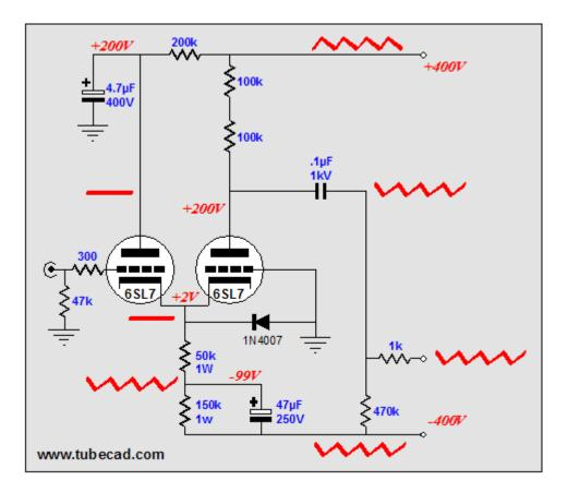
Is the common-cathode amplifier the only topology that allows us to inject the negative power supply rail noise into its output? No, as several other topologies can be "fixed" to achieve the same end, starting with the insanely ubiquitous grounded-cathode amplifier. (Imagine that this topology were made illegal; what would 90% of tube gurus do?)
