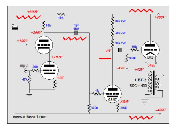
Using a pentode-based input stage, with the same power supply decoupling, would also yield the desired result.
