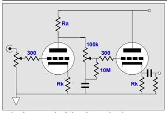
In the second of the above circuits, we see a series attenuator bridging the input groundedcathode amplifier to the output cathode follower. Because the attenuator terminates into a shorting capacitor to ground, the DC voltage relationships remain constant no mater what the attenuator's setting.
