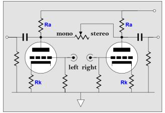
But the cathode resistor should be left unbypassed, as an unconstrained cathode will be needed to implement the broadening of the signal. With the unbypassed cathode resistor, the resistor value for 50% must equal:
