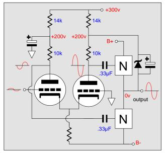
Eliminating the noise is a bit different in this circuit compared to the no-gain version. As shown below, the power supply noise grossly amplified by the top output device. Here the cathode resistor relays the negative rail noise to top device's input where it is greatly amplified.
