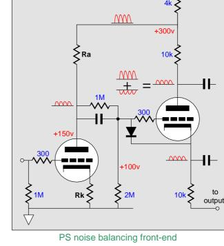
If a pentode or FET is used as the input tube, then a 50% voltage divider is needed. Two equal valued resistors will work. The trick will be to find the value for these resistors that is not so low as to excessively load the first stage and not so high as to limit the high frequency response of the signal leaving the split-load phase splitter. Understand that this voltage divider will also divide the audio signal from the first tube. Still eliminating noise often comes at a price.
