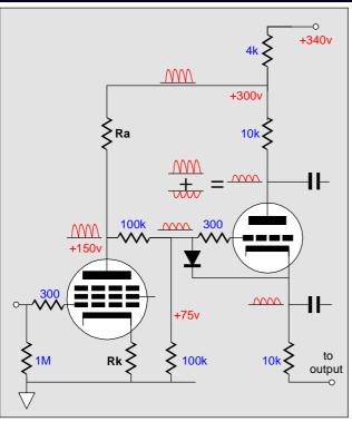
Pentode front-end with a resistor voltage divider
