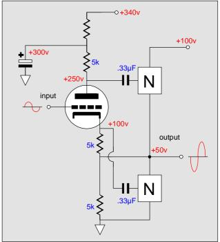
Split-load, cathode-referenced, gain output stage
