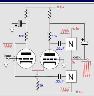
Replacing the cathode resistor with a constant current source, once again, does not eliminate the noise, but interestingly it does not invert the phase of the noise at the output.
