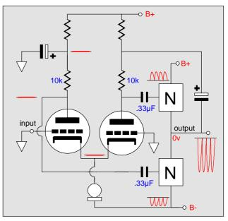
Keeping the current source and shifting the power supply filtering capacitor's termination from ground to the negative power supply rail (as shown below) is the trick to eliminating the noise. This is another example of how the whole circuit, the driver circuit and the output stage and the power supply, must be analyzed to fruitfully design a power amplifier.
