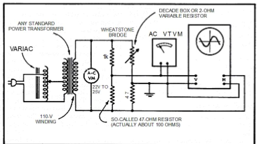
Fig. 1. Test circuit used to demonstrate non-linearity of the offending resistor.
